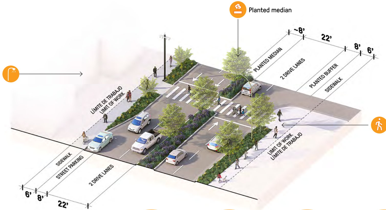
FIGURE 4.24 SANBORN ROAD AND MOHAR ST INTERSECTION - AXONOMETRIC Proposed planted median and crosswalk at Breadbox Recreation Center
