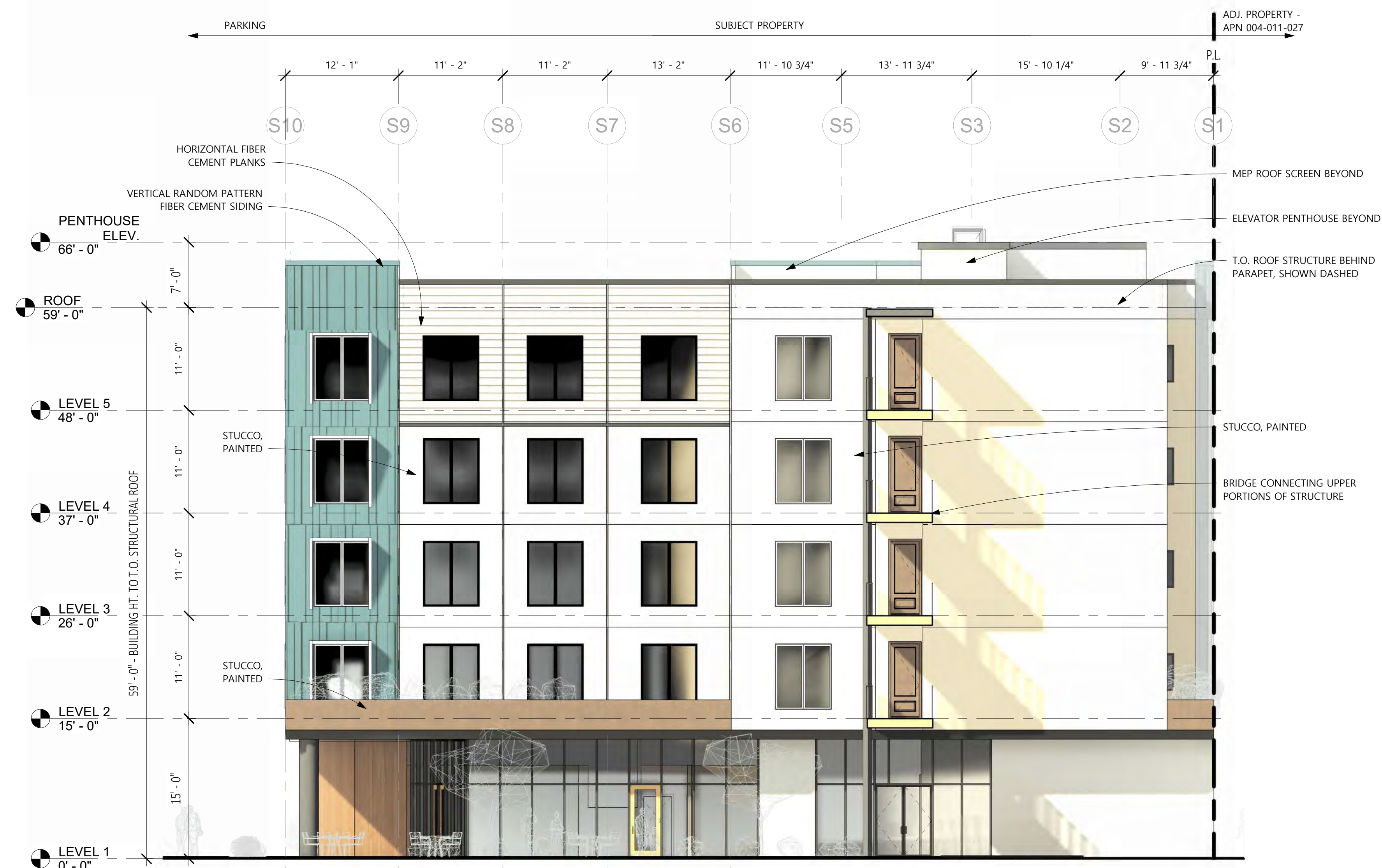
① SOUTH BUILDING WING - NORTH ELEVATION 1/8" = 1'-0"
