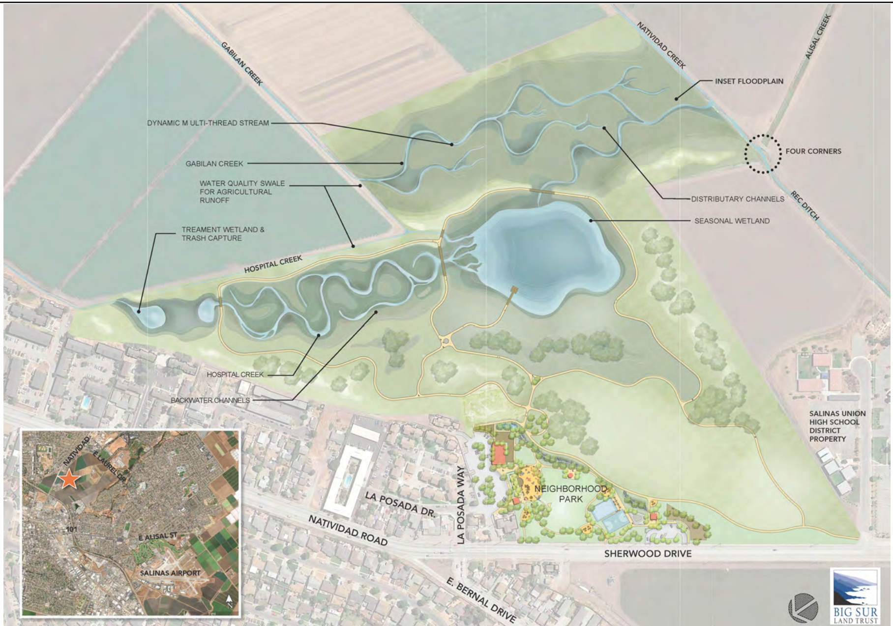
Figure 2. Concept Sketch Incidental Take Permit No. 2081-2022-027-04 Carr Lake Restoration and Park Development Project
