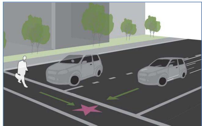
Multiple threat conflicts on multi-lane roadways occur where a vehicle yielding to a pedestrian inhibits sight lines to another oncoming vehicle.
