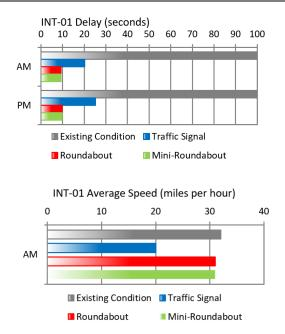
The bar chart to the left compares the peak hour intersection delay for design year between the existing control and each of the proposed intersection control alternatives.
