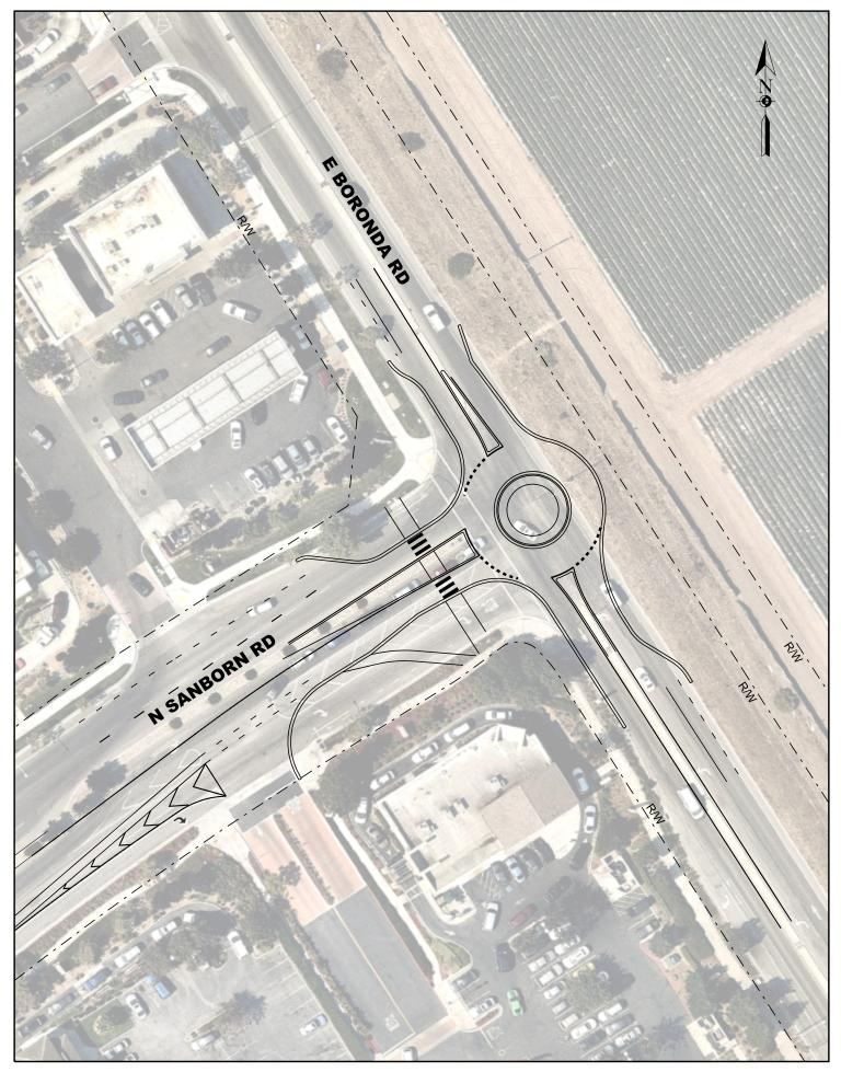
Kimley»Horn E BORONDA ROAD AT N SANBORN ROAD ALTERNATIVE C: MINI-ROUNDABOUT
