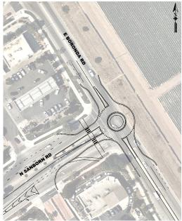
Figure 4: Mini-Roundabout Control
