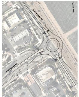
Figure 3: Single Lane Roundabout Control
