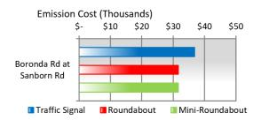
Both roundabout and mini-roundabout alternatives are preferable to the traffic signal when based solely on fewer tons per year of mobile source pollutant emissions and the societal cost associated with exposure to these health based pollutant emissions. The figure shows the emission cost of year 2018 based on the average speed through the intersection with each intersection control types.
