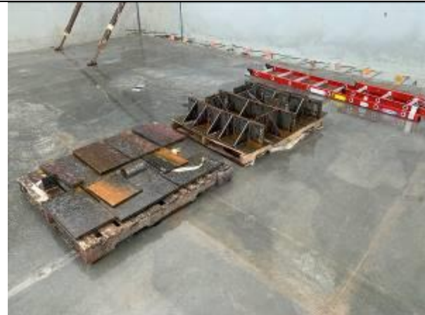
Steel connector plates for wall connections
