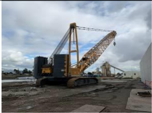
Crane used to lift wall panels
